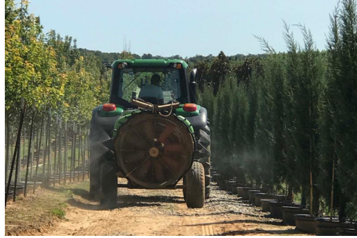
One version of the intelligent sprayer. (photo by Amy Fulcher, UTIA)
