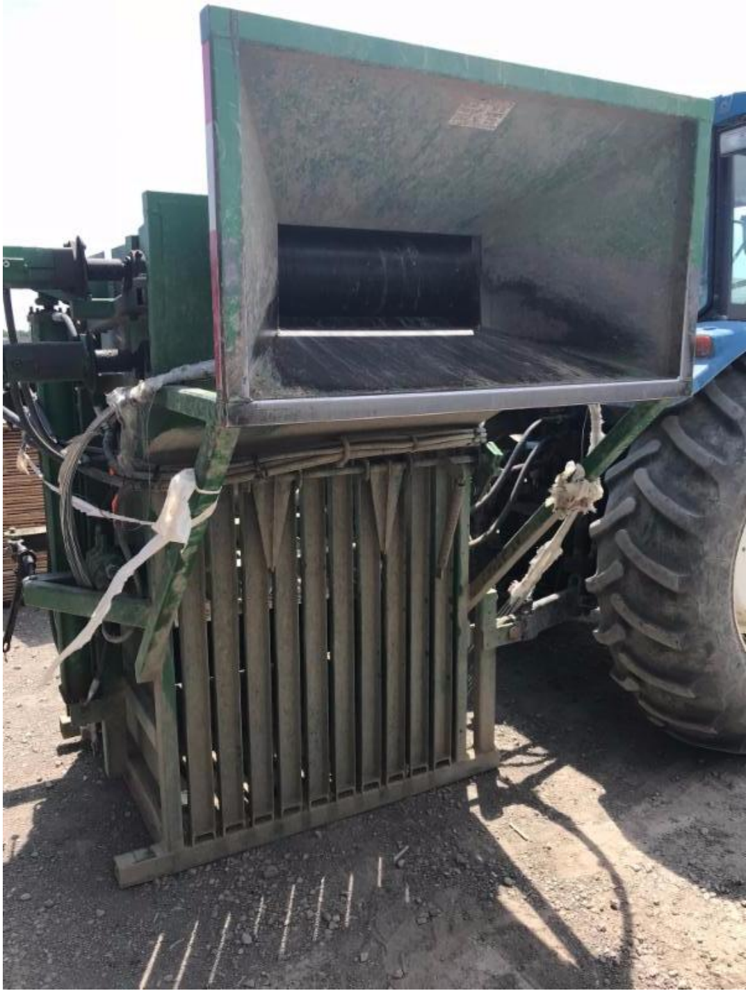
Plastic bailer for removing and compacting plastic.
