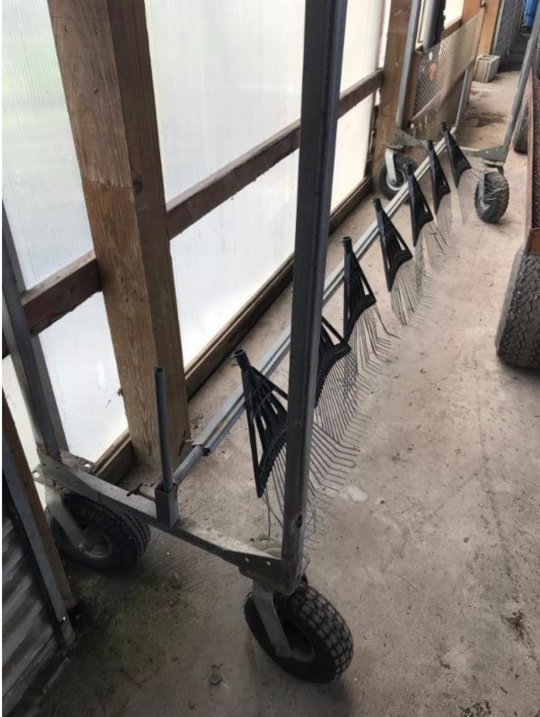
Rake push cart used to knock off granular herbicides from leaves.
