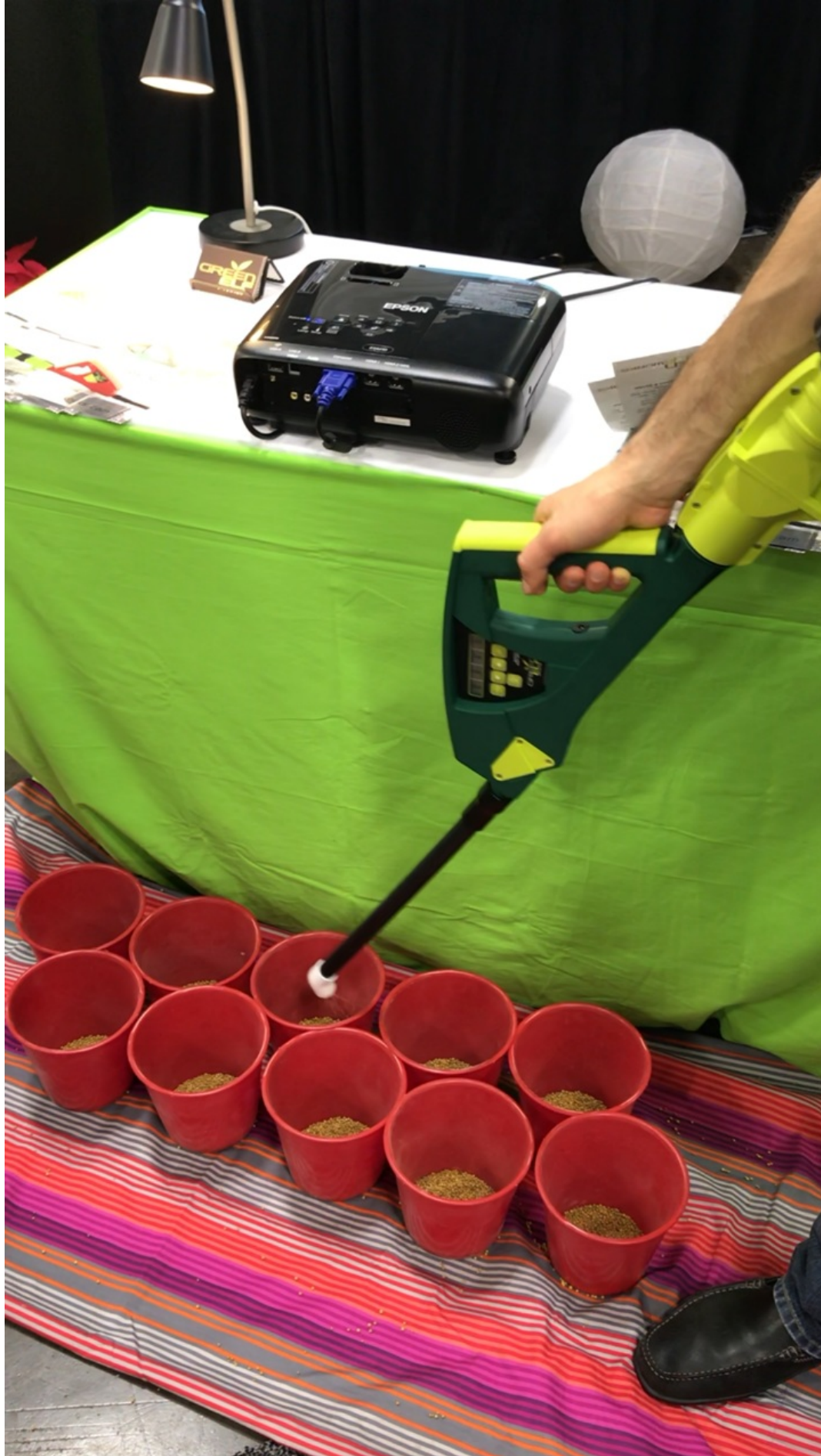
Granular topdress applicator (models for fertilizer and herbicide).
